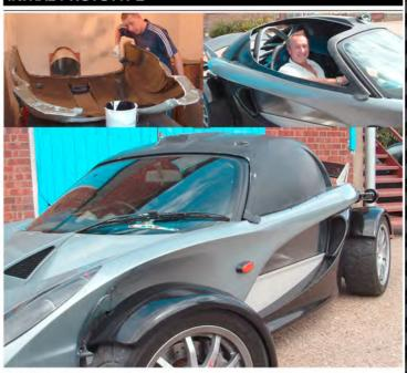
A GRP prototype tool was made from the hardtop pattern with no door gutters. A part was made from the tool & successfully trialled & fitted to a 340r. The door aperture was then cut & access tested.
