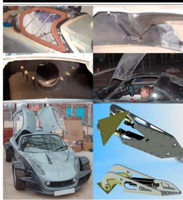
Gutter returns were modelled in clay to allow modification of the tool. A centre spine was produced combining centre roll hoop fixing & ram-air induction. A dihedral door system was selected & an initial prototype hinge was produced. This was CAD modelled to be produced in machined alloy.
