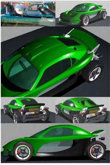
Initial sketches were made of 3 roof style options. After selection of the version to develop, the complete surface of the 340r main body, roll bar, & screen surround was modelled in CAD along with the hardtop. Comprehensive measurements were taken to allow accessibility for tall drivers with crash helmets (for track day use). Details such as the rear screen, package design & ventilation were looked at in detail.
