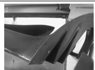
58mm (R01SE0009) & 75mm (R01SE0178) Exit Naca Ducts, angle trimmed on exit to remove snorkel & bonded under 340R Front Spoiler, Deep Version.
