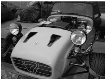
2x 75mm Exit Naca Ducts (R01SE0178) fitted to Caterham SV nose cone.
