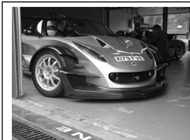
340r Featuring reverie deep front spoiler (R01SB0051). The spoiler has then been modified underneath with Naca ducts as the image on the RHS shows to diffuse the air into the wheel wells, aiding front downforce by making the splitter work more effectively.
