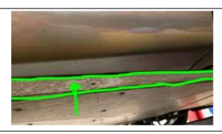
4. Fit self-adhesive EPDM sponge rubber 50mm x 2mm strips 1.65m long to each outer side aluminium chassis strip to stop corrosion between the carbon sill top and aluminium chassis, then remake the holes through the foam
