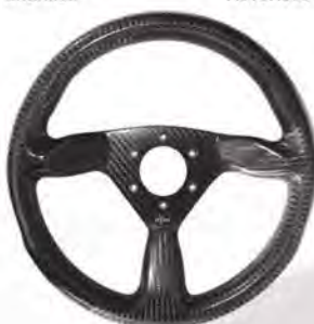
Eclipse 315 optional 23mm mounting offset, approx mass: 255g
