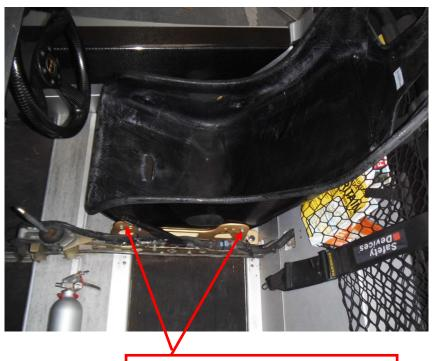
once the subframe bolted tight to the floor pan then the subframe can be tightened to the seat.
