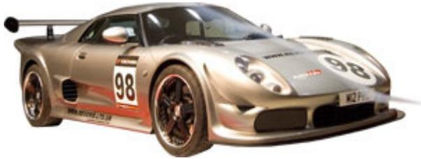
**Our last test yielded the best results with only a 10% increase in drag but gaining 56% extra overall down force. We also moved the down force distribution (overall balance) from 9% on the front to 38.5% on the front giving a 38.5% - 61.5% front to rear distribution.**
