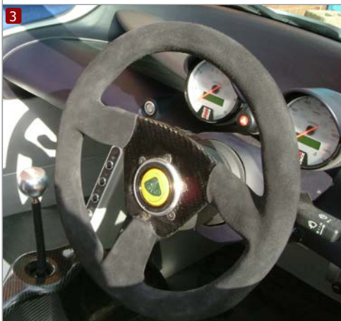
23mm offset drilled in Lotus 340R
