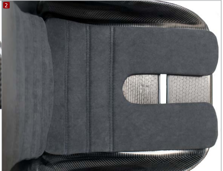
Velcro fitting for quick fitting/removal
