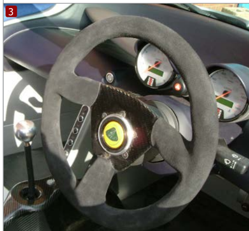
23mm offset drilled in Lotus 340R
