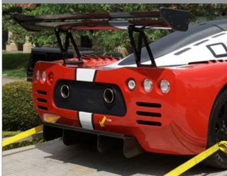
3 element diffuser on Ultima GTR
