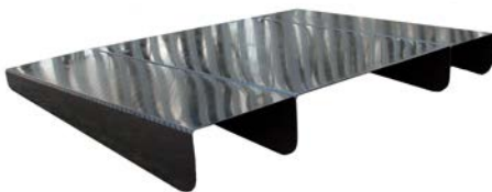
Joined diffuser tunnels
