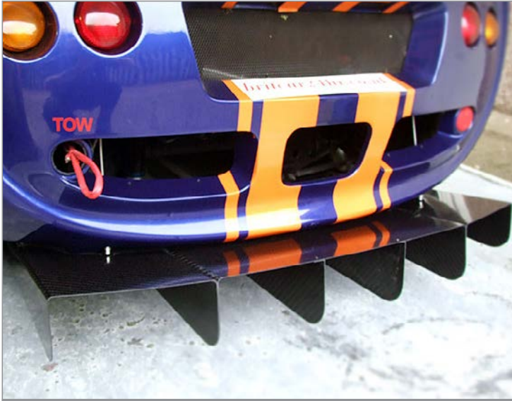
5 element diffuser on Lotus Exige S1
