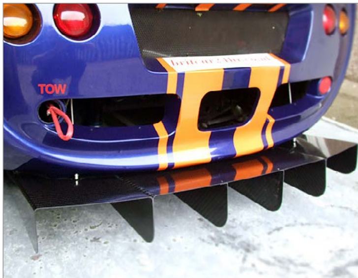
5 element diffuser on Lotus Exige S1
