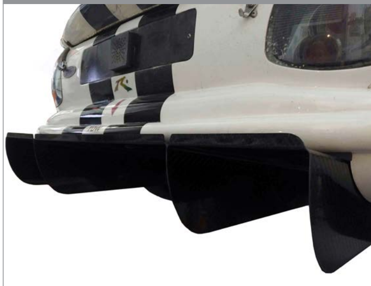
3 element rear diffuser on TVR Cerbera
