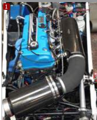
Caterham 7 with Honda B20 engine with Interlagos 112D LH
