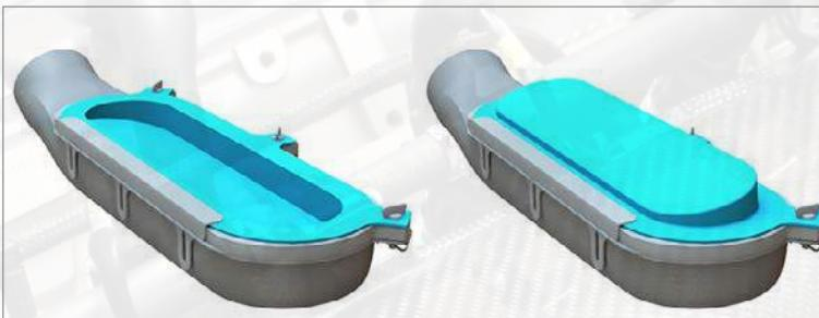
30mm back plates can be reversed to fit into the air box to allow for reduced air box depth (see image, left) which may be required if fitting in restricted engine bays. On some setups, this would be required if the air box foul's fuel rails/injectors. An example of this can be found on our Morgan Omex Throttle body induction kit. Where this is used, an external remote filter is required and you will likely need to use short ram pipes/trumpets to allow 25mm minimum clearance - 40mm ideally.
