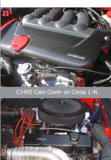
C14XE Cam Cover on Corsa 1.4L
