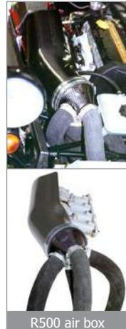
Noise reduction is increased when using multiple smaller intakes and our Porous sound absorbing ducting. Multiple smaller size inlets can additionally allow for some bottom end torque tuning or oval inlet pipes could be used to create a comparable open area. High flow alloy straight trumpets can also be used as intakes.
