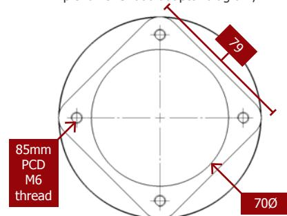
A bolt-on 64 to 70mm tapered bore adaptor is also available (R01SE6182)
