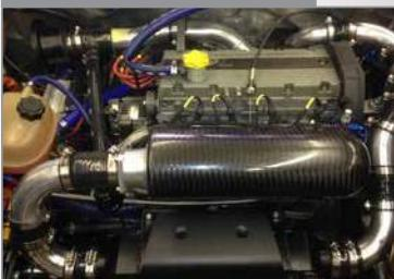
Fontana 112 on Rotrex supercharged K-Series engine
