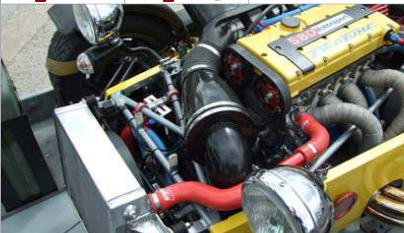
Daytona 230 remote filter setup on Caterham 7 with C20XE engine
