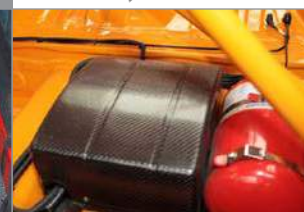
FIA Battery Box in BTCC
