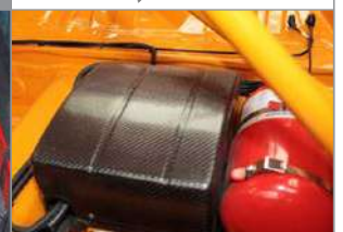
FIA Battery Box in BTCC
