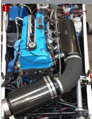
Caterham 7 with Honda B20 engine with Interlagos 112D LH
