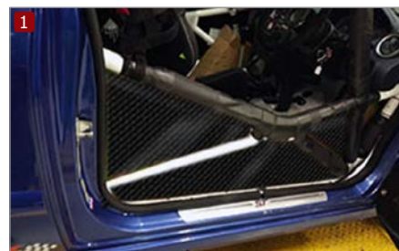
Alloy honeycomb roll cage door bar impact protection panel/sheet. Required in many saloon classes and BTCC touring cars.
