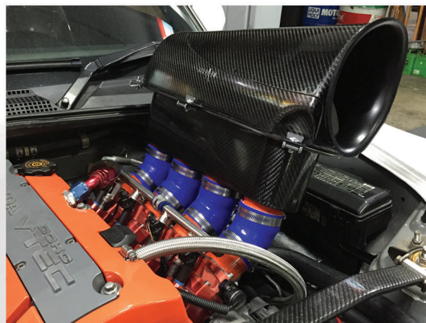
Zolder 150 on Honda S2000 with 127mm alloy inlet trumpet
