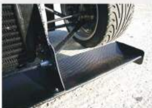
Caterham CSR/Levante/SV front wing assembly 1285mm wide with end plates M02SB0010 (Std S3 Chassis: M02SB0013)
