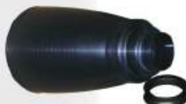
Daytona 230 TT filter canister, shorter than standard Daytona 152mm inlet, 100 / 75 / 58mm outlet for use with Reverie cone filter Filter flows 166 cfm at 1.5" H 2 O using 100mm inlet/outlet
