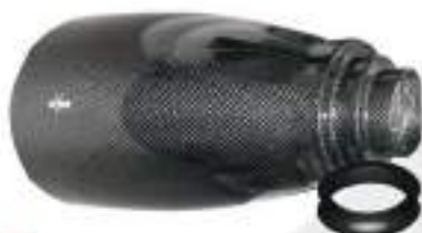
2 Daytona 230 carbon fibre canister, 152mm inlet, 100 / 75 / 58mm outlet for use with bespoke to Reverie cone filter Filter flows 166 cfm at 1.5" H 2 O using 100mm inlet/outlet
