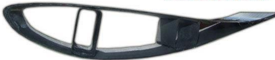
300mm Chord Wing Showing Internal Longitudinal Stringers
