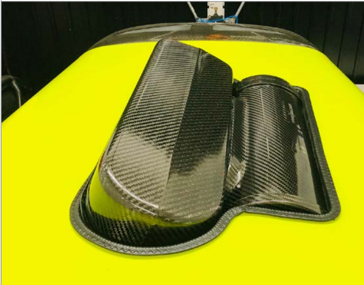
Height of air filter box can be customised to go under or fro more volume through the bonnet as shown
