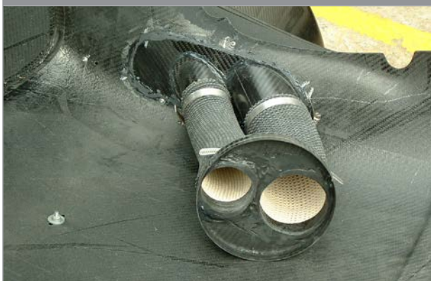
58mm and 75mm Snorkels bonded inside single Blister nose to Daytona 6" filter adapter for Ram air
