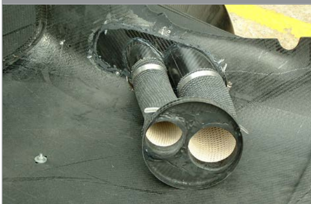
58mm and 75mm Snorkels bonded inside single Blister nose to Daytona 6" filter adapter for Ram air
