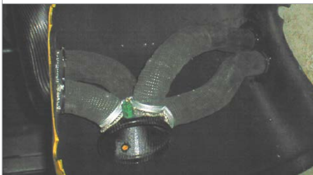
4 off 58mm snorkels inside a pair of Blisters to 4 way 58mm 6" filter adapter for Ram air
