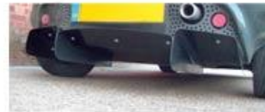
Exige with Reverie 111S diffuser and high exit exhaust with 3 centre tunnel and two side fixing holes
