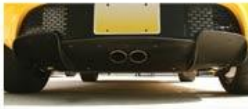
Standard diffuser shown with 5 rear centre tunnel fixing holes and 3 side fixing holes
