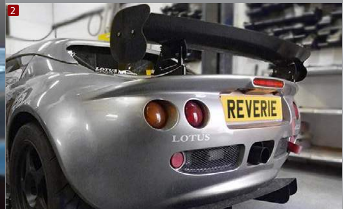
Adjusted by the four rose jointed carbon support posts
