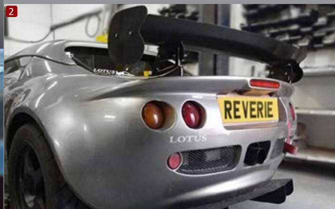
Adjusted by the four rose jointed carbon support posts
