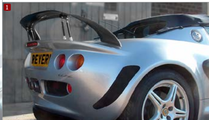
Adjusted by the four rose jointed carbon support posts
