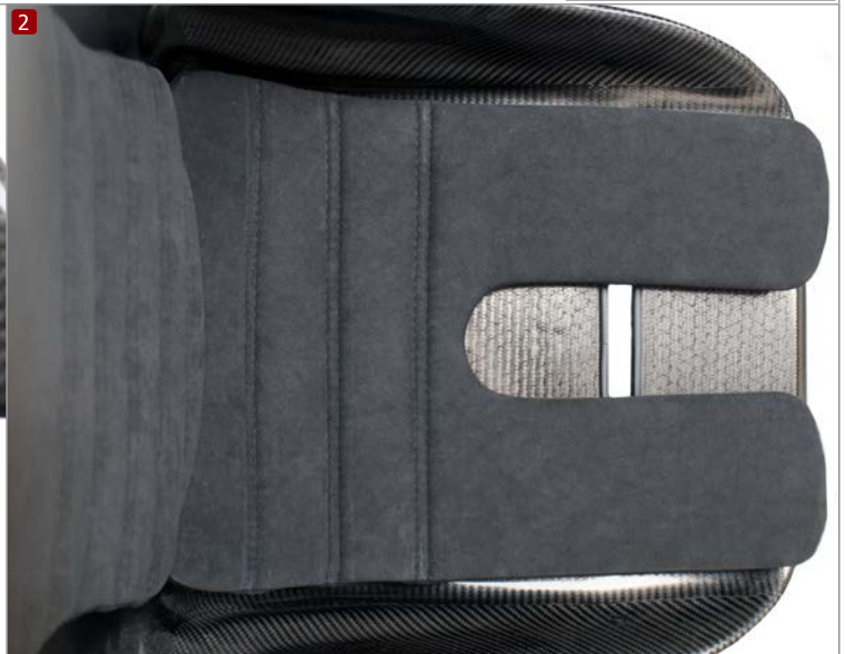
Velcro fitting for quick fitting/removal
