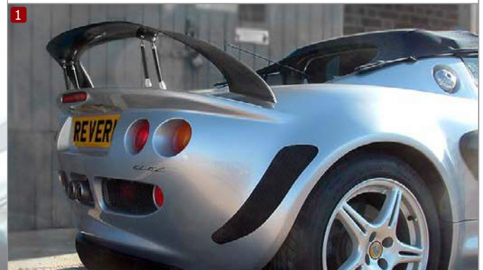
Adjusted by the four rose jointed carbon support posts
