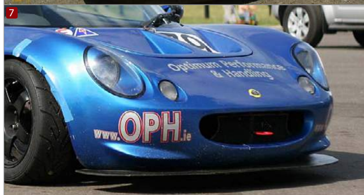
Carbon Fibre front spoiler increases down-force reducing front end lift at high speeds. Available painted to the colour of your car at extra cost
