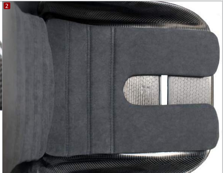
Velcro fitting for quick fitting/removal
