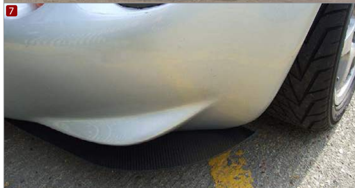
Carbon Fibre splitter plate that can be used with or without front spoiler. Provides additional down-force by improving air flow underneath the car
