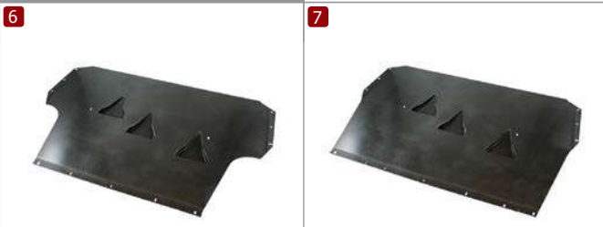
Can be supplied without NACA ducts (advise when ordering) Increased width floor section for use with diffuser 12
