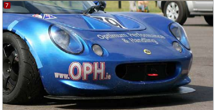
Carbon Fibre front spoiler increases down-force reducing front end lift at high speeds. Available painted to the colour of your car at extra cost
