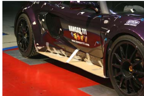
8. Horizontal side sills simulated
