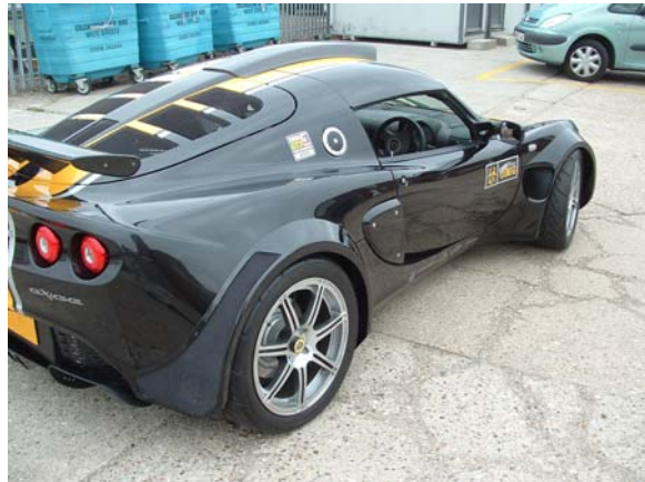
Car 001 GT3 Exige Cadena 2006 Replica with ReVerie Vented Arches To reduce high pressure build up and hence lift under arches
