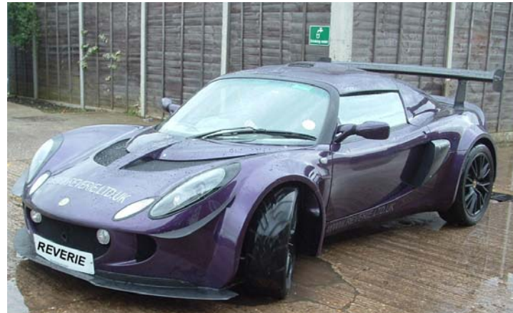
Tested Exige S2 with blended in ReVerie Wide Arch kit Wing shown in pre-test 223mm position. N.B Car not fitted with wide mid floor, horizontal side sill fences or longer diffuser
