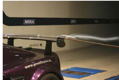
Vortex's generated by end plate design
