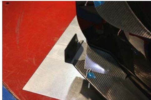
8. Side Fences fitted to front spoiler
