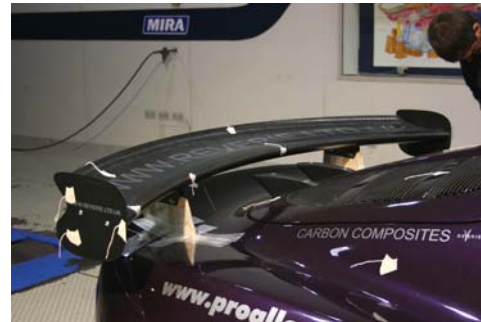
5. Rear wing lowered to 93mm 10' AOA
