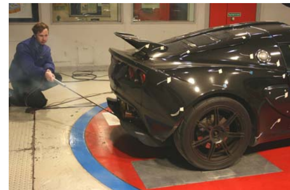
Left Image: Stalled flow in side diffuser tunnels Due to no floor / diffuser under rear wishbones Right Image: Good flow in centre tunnel as exhaust Exit above diffuser and 111s style diffuser fitted.
