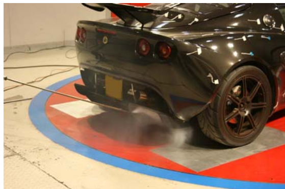
Left Image: Stalled flow in side diffuser tunnels Due to no floor / diffuser under rear wishbones Right Image: Good flow in centre tunnel as exhaust Exit above diffuser and 111s style diffuser fitted.
