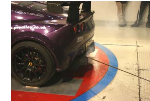
Disturbed rear diffuser centre tunnel flow by exhaust
