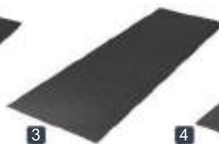
2 ply carbon fibre sheet 0.55 mm thick
