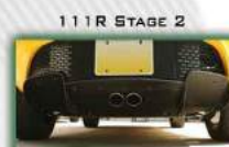
111R STAGE 2 5 rear centre tunnel fixing holes and 3 side fixing holes
