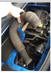
3. Carefully break the cable ties and remove the Two porous intake hoses from the lower airbox as shown
