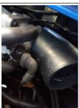
Remove the original rubber intake below hose and fit the new Daytona rubber connector elbow with hose clip to throttle body, with the outlet pointing slightly down and rearwards
