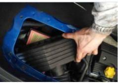
1. Unclip the four clips around the Airbox lid and undo the retaining jubilee clip to the rubber below intake hose, remove air box lid
