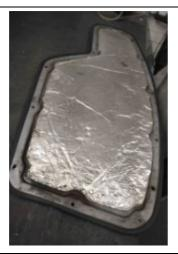
Inside the MG on the rear parcel shelf, undo the clips retaining the rear of the hood down. Then lift the rear of the convertible hood and rear window up and unbolt and remove the top engine access panel.
