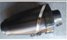
4. Fit the Filter inside the Daytona canister and the filter adapter then inside the filter and carefully secure both the hose clips around the filter neck
