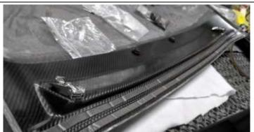
7. Front latch clip view to align with clips to fit to front windscreen roll hoop
