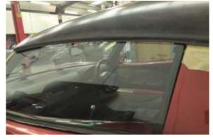
8. Side view of roof fitted to car the side windows may need height and door angle adjustment to best fit also the rear buttress height can be adjusted with foam packers if needed each side.
