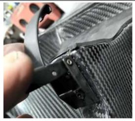
5. Rear hard top Roll hoop retaining latch one each side, remove the standard roll hoop cover first
