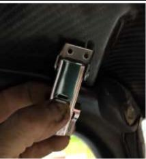
9. Front catch location images, customer fits the latch point to his front screen surround with rivets to supply
