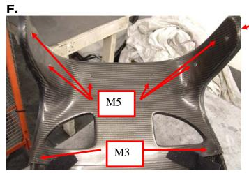
YOU CAN NOW BOLT THE HEAD RESTRAINT HALVES TO THE SEAT WITH THE FASTENERS PROVIDED
