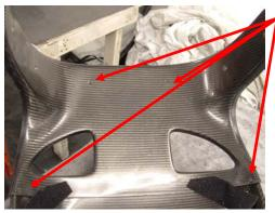
WITH A MARKER PEN (A WHITE PAINT PEN IS IDEAL) MARK THROUGH THE FOUR HOLE'S INDICATED ON TO THE SEAT. REMOVE THE HEAD RESTRAINT FRONT AND PILOT DRILL WITH A 3mm DRILL BIT THROUGH THE SEAT WHERE MARKED.
