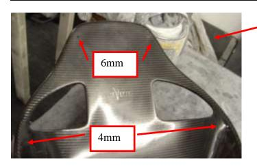
THE PILOTED HOLES SHOULD NOW BE OPENED UP TO THE INDICATED DIMENSIONS
