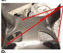
WITH A MARKER PEN (A WHITE PAINT PEN IS IDEAL) MARK THROUGH THE FOUR HOLE'S INDICATED ON TO THE SEAT. REMOVE THE HEAD RESTRAINT FRONT AND PILOT DRILL WITH A 3mm DRILL BIT THROUGH THE SEAT WHERE MARKED.
