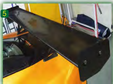
5 Exige V6 Carbon Fibre 310mm High Downforce Clam Mounted Adjustable Wing R01SB0472
