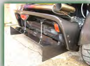
Standard length diffuser fitted
