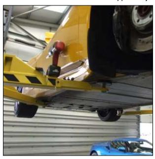
2 Remove existing side sills from vehicle. The side sills are held on by 4x M6 screws (2 at the front, 2 at the rear;
