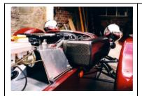
6. Bolt the backplate to the carbs/throttle bodies with the inlet trumpets in place. Refit the airbox and ensure there are no foul conditions. Where an airbox protrudes through the bodywork small amounts of trimming might be required if the airbox is larger than the previous filter.
