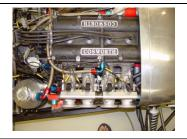
1. Remove existing airbox/air filter from the engine and leave trumpets attached to throttle bodies/carbs.
