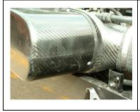
9. The airbox can now be semi-permanently attached to the backplate. Use thread sealant on all the bolts and screw into place so that they are all hand tight. With the airbox in place it is now possible to route ducting to it from a remote filter, filter canister or intake scoops (where trumpet socks have been used). The deep threaded Unuts and fixing holes can be moved to wherever is most appropriate for best access as shown (positions provided in factory items are only for guidance).
