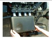
2. Offer up the airbox without its backplate to check for clearance. It is possible that the airbox may require some trimming to fit within the constraints of the engine bay. Use of a template might make visualisation of this easier. Once happy that sufficient space is available bolt the airbox to the backplate ready for the next stage of fitting. Note that there should always be at least a 25mm gap between the airbox and trumpet mouths.
