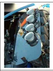
The flat backplate airbox kits are supplied with angle brackets to allow fixing of the backplate to the airbox. The angle brackets can be permanently attached to either the backplate or the airbox by use of an epoxy adhesive and a single rivet to maintain its position during cure. Shown here are brackets attached to the backplate.
