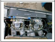
3. Remove the airbox and fit the deep threaded U-nuts to the angle brackets. If necessary the hole in the angle bracket can be slotted and the U-nut placed on the side of the bracket so that it can slide up and down allowing the box to be pushed home hard. When happy with the seal, hand tighten the bolts. The airbox shown here has the brackets bonded and riveted to the airbox and relies on the bolts to pinch the seal.
