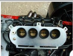
1. Remove existing airbox/air filter from the engine, having first removed air temperature sensor and breather pipe.
