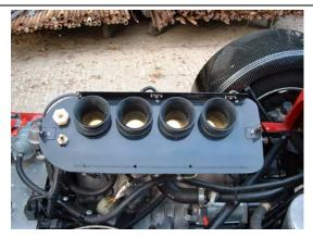
3. Fit composite back plate with trumpets to throttle bodies. Note offset nature of back plate trumpet grommet section alloys back plate to be offset if required by turning trumpets in back plate. Refit temperature sensor and oil breather.
