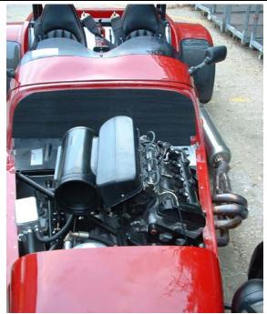
4. You are now ready to screw the air box in place. Use the bolts supplied, if we have supplied the airbox with aircraft anchor nuts these are self locking. These fixings have a 2.5mm rivet either side to secure them in place. If we have supplied the airbox with clip over deep threaded u-nut fixings then you must use a thread lock to ensure the bolts do not come loose. Push the airfilter with extension moulding into end of suzuka tube and secure with single hose clip supplied.
