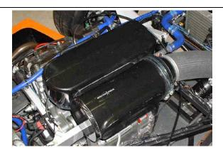
6. If cold ram air is required then at optional expense a flat or stepped diffuser cone, trunking and an alloy intake bell mouth or scoop can be fitted. See <a href="https://www.reverie.ltd.uk">www.reverie.ltd.uk</a> for details.
