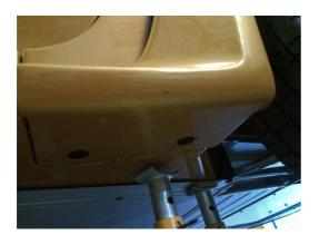
4. Fit the 2 off M6 c/sunk 40mm bolts and bevel washers in place of the lotus front fender lower bolts. Do this on both sides of the car. Once happy drill through into the GRP sill carefully! (oil pipes present!) through the additional holes in the panel, use a 4mm then a 9mm drill bit..
