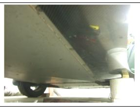
3. Support the front of the carbon sill up on blocks against the chassis and adjust it so it fits and looks even.
