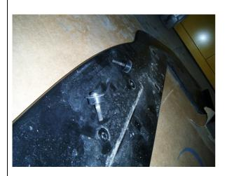
4. 2 Front centre bolts with spacers, spacers which must be retained and re used on rear of centre forward holes.
