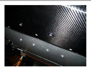
6. Use C/sunk Alloy Bevel washers supplied on the two front centre holes which have the spacers on the rear and M6x30mm bolts. Then use M5 x 30mm and 2 countersunk bevel washers on the one hole either side at the front.
