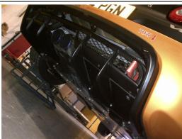
2. Unbolt the OEM ear diffuser to allow access to the Rear upper diffuser surround trim bolts and rivets.
