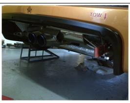
4. Now unbolt the one lower bolt each side and the 5 upper bolts and carefully drill out the upper diffuser surround fixing rivets. Also remove any parking sensors if fitted, these cannot be refitted to our Reverie part (unless you do your own custom modification).
