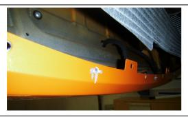
7. Now you need to fit the supplied anchor nuts where the original top 5 bolt holes were. Drill counter sunk rivet holes and fit the anchor nuts on the back of the fibreglass suing 2.4mm c/sunk rivets supplied.
