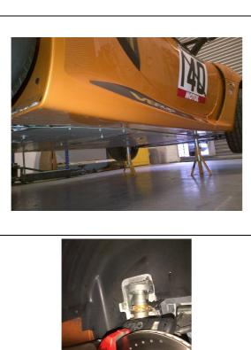
1. Handbrake on, Loosen front wheel nuts using locking wheel nut tool and torque wrench etc.
