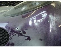
4. Offer front canards in position and drill four 5.5mm fixing holes each side.
