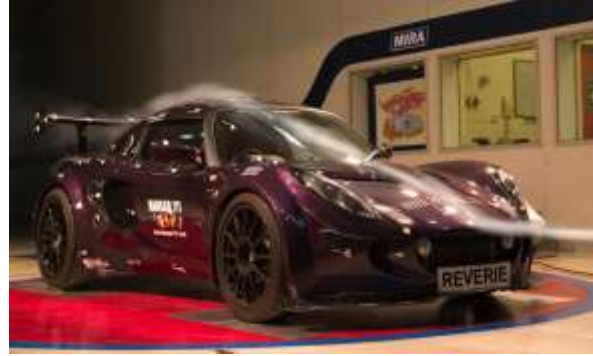
Similar Exige Based Wind tunnel Testing
