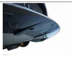
5. Loosely bolt the spoiler up and centralise it on the car till best fit achieved and then bolted in place. Once happy with fit stick the supplied black 50mm diameter stickers over the large holes on the underside to reduce drag.
