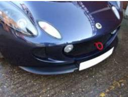
2. Remove standard front spoiler and number plate from old spoiler. Also remove the bolt at the centre of the vehicle just behind the spoiler that bolts the clamshell to the alloy floor panel.
