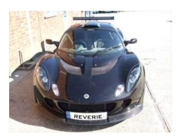
7. Hold the front number plate in position and drill a 5.5mm hole either side through the plate and into the clamshell. Then Fit M5 rivserts into the clamshell and bolt the number plate on as shown, you will need to slot the number plate holes a little across the car to allow for the angle the bolts will go in at on the radius. Refit and torque wheels if removed and carefully lower to the around.
