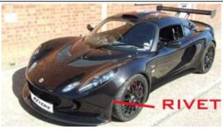
6. Drill and rivet through the spoiler where marked into the clamshell and fit 4mm peel rivets. Paint heads of rivets black.
