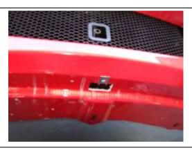
4. Drill the additional centre hole front to 6mm (as marked in step 3) and then dremel the slot in the clamshell to allow the M5 deep threaded u-nut to be fitted. Bolt the spoiler up into position with the larger than stock newly supplied 25mm diameter m5 washers.
