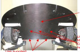
Use supplied M5\*30mm bolt with 13mm Spacer and C/Sunk washers here, 1 off
