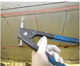
4. Drill the additional holes at the rear of the spoiler into chassis 7.2mm (as marked in step 3) and then inset the 3off M5 rivserts with a nutsert or rivsert tool
