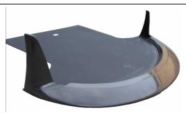
3. Position new front spoiler in place, best to have 2 persons so as not to damage clamshell. Mark through the spoiler for the additional hole in the rear of the part.
