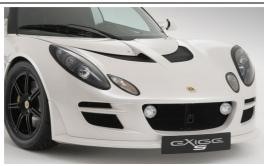
2. Remove standard front spoiler and number plate from old spoiler. Also remove the bolt at the centre of the vehicle just behind the spoiler that bolts the clamshell to the alloy floor panel.
