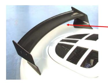
WE RECOMMEND SETTING THE WING TO BETWEEN 8 AND 12 DEGREES AOA AS A STARTING POINT, PLEASE DRIVE ON TRACK SENSIBLY AND TUNE AOA UNTIL A NICE BALANCE POINT IS FOUND.
