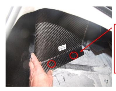
DRILL AND ATTACH CLAM SUPPORTS TO THE CLAM IN BOTH SIDES USING EXISTING FITTING HOLES FOUND IN THE CLAM USING SHORT SCREWS FOUND IN KIT. YOU MAY NEED TO MOVE THE BATTERY.
