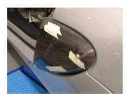
5. New reverie outer duct shown ready to be fitted, use longer bolts supplied (45mm under head) and 20mm spacer upper forward, 7mm spacer rear, 25mm lower forward. You can adjust post length by sanding or adding washers if required for car to car tolerance variations. You should refit the O.E rubber washer and then nylon washer after the spacer posts to hold everything on the bolt whilst you are trying to position and tighten into place.
