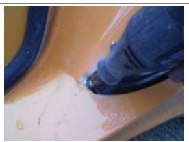
4. Drum sand using a dremel with 80 or 120grit abrasive drum sanding bit. Also use a diamond point 3mm dia to get the harp beak point required.
