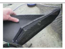
3. View of new side duct showing protective rubber edge strip
