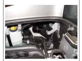
9. View of the scoop under hood, ready to be connected to 111r Daytona induction kit.
