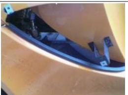
4. Fit 400mm long dx85 u-section rubber supplied (each side) over lower lip of bodywork to hide poorly trimmed factory panel edge. Do not fit this rubber if you are fitting the optional inner duct.
