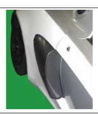
4. Optional outer carbon side ducts shown. N.B with holes for Exige S2, without holes for Elise S2. See <a href="www.reverie.ltd.uk">www.reverie.ltd.uk</a> for details. Refit the inner wheel arch liners and refit the road wheels. Lower car to the ground and torque wheel nuts.
