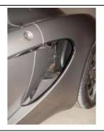
Chock front wheels, Jack up rear of car and remove road wheels. Remove the rear inner wheel arch liners and standard plastic side duct.
